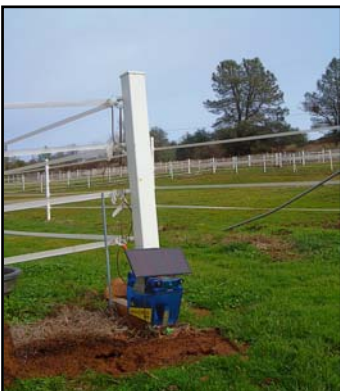
Solar fence charger with electric web fencing for interior fencing
